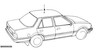
After drilling the hole for the antenna remember to clean the hole from the drilling swarf, so that surface is even. This is needed in order to ensure proper and reliable connection between the ground plane and the antenna. After cleaning it is advised to apply some rust–proofing compound to the hole.
